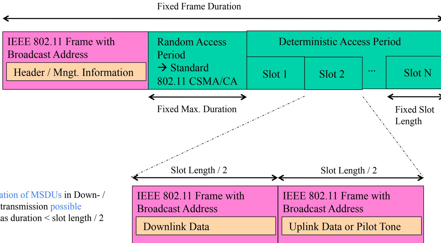
Aggregation of MSDUs in Down- / Uplink-transmission possible as long as duration < slot length / 2
